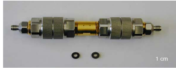
Fig. 2. Test fixture for transmission–reflection measurements of cylindrical hexaferrites.
